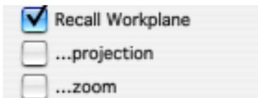
Upon selecting a WE in the palette menu, these 3 checkbox show which information is going to be updated in the current view. If only the WP position is checked, then only the WP position recorded in the WE menu is called back. The projection type can also be recalled (plan view, axonometric, etc.) and the zoom frame, that is the zoom position and scale. These 3 informations are independant and usable as such.
